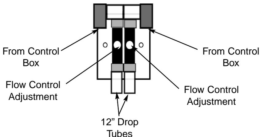
The flow control valve meters the volume of air escaping from the bottom of the cylinder as the piston is being pushed downward. Closing the valves will slow the travel speed of the door. The check ball in each valve allows each cylinder to breath freely as the piston is draw up mechanically by the chain on the reverse cycle.
