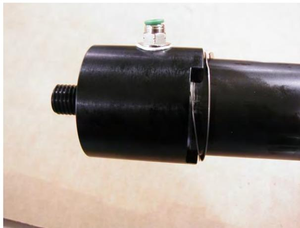
Step 10 – Re-mount cylinder into brackets and tighten mount nuts and lock washers. Re-couple cylinder by pressurizing the piston end of cylinder which will drive the piston towards the carrier. Increase pressure until a distinct noise is heard which indicates coupling. Check that the end of carrier is approximately 1/8 inch from cylinder head. Cycle cylinder to other side and check the same distance, if both ends match coupling is complete.
