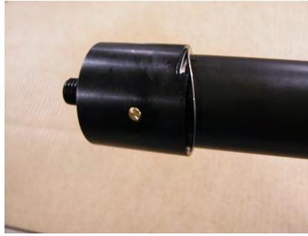
Step 2- Remove head from cylinder tube by pulling head directly away from tube. Remove retaining ring from cylinder tube. **Be careful not to damage head o-ring and not to deform retaining ring.**
