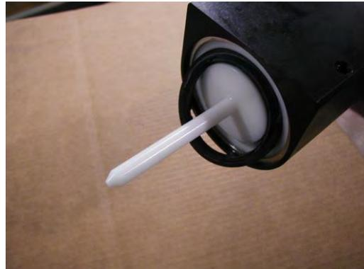
Step 5 – Remove the piston from the bore of the cylinder making sure to mark direction same as carrier. Remove piston bearing ends by holding one and rotating the other CCW to unthread from each other. Replace both piston ends with new ends provided. Install new piston o-ring seals on each piston end. Lubricate o-rings Magnalube-G grease.
