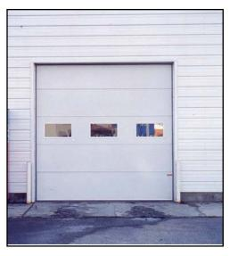
Our 3" Sections are roll-formed from hot-dipped galvanized commercial quality steel. The exterior and interior skins are 26 ga. pebble textured steel, pressure-bonded to an extruded, closed-cell polystyrene which has minimal moisture absorbsion qualities unlike expanded polystyrene (bead-board) type products.
