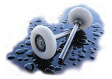
Magnum **Supreme Rollers Double-Sealed Precision** Bearing: **Ball Bearings: Stainless Steel Raceways: Stainless Steel** Tire: **UHMW Polvethvlene** Tire Face: **Shielded Inner Face** Stem: **304 Stainless Steel** Collar: **304 Stainless Steel**
